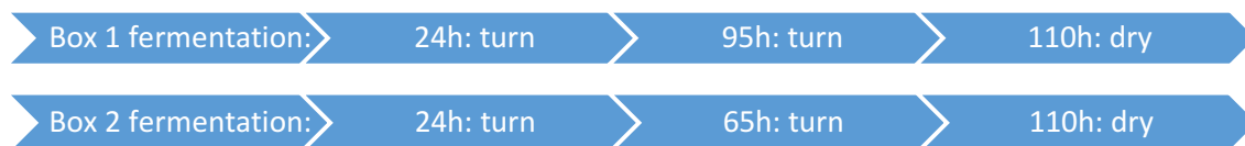
Figure 5: turning frequency employed for the two fermentation batches. Box 2 was turned earlier as the temperature had not reached 45 °C after 48 hours
