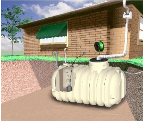
Fig. 4.1: Underground Rainwater Tank Source: www.rainharvest.co.za/
