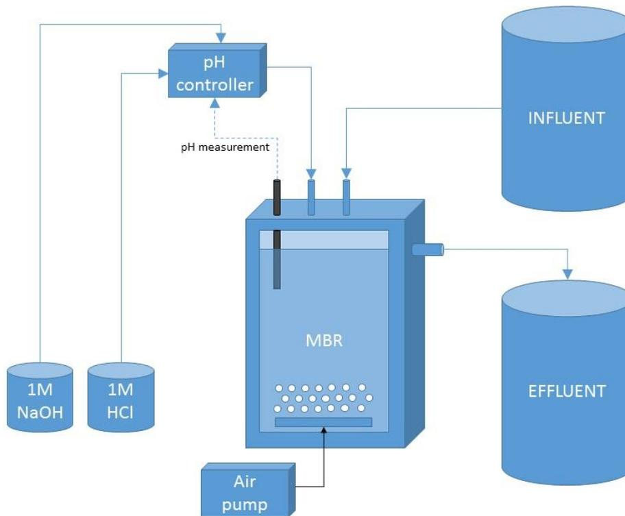
**Figure 8: Setup of the membrane bioreactor (MBR). Influent and effluent flow rates are regulated by a peristaltic pump coupled to a timer (not depicted).**
