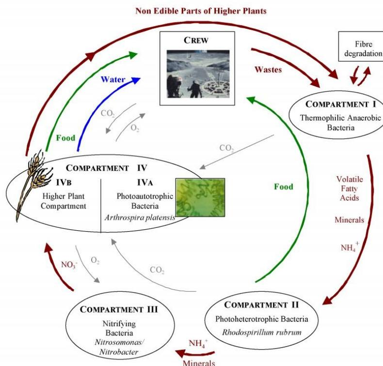
**Figure 1: Scheme of the MELiSSA loop (Micro-Ecological Life Support System Alternative). Figure from Hendrickx et al. 2006**
