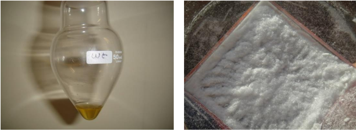
Figure IV.15: Demonstrating the necessity of enzyme engineering: with the wild type, no crystallization was observed (left), while crystals with a high purity (> 99.5 %) were obtained with the BaSP_L3411_Q345S mutant (right).
