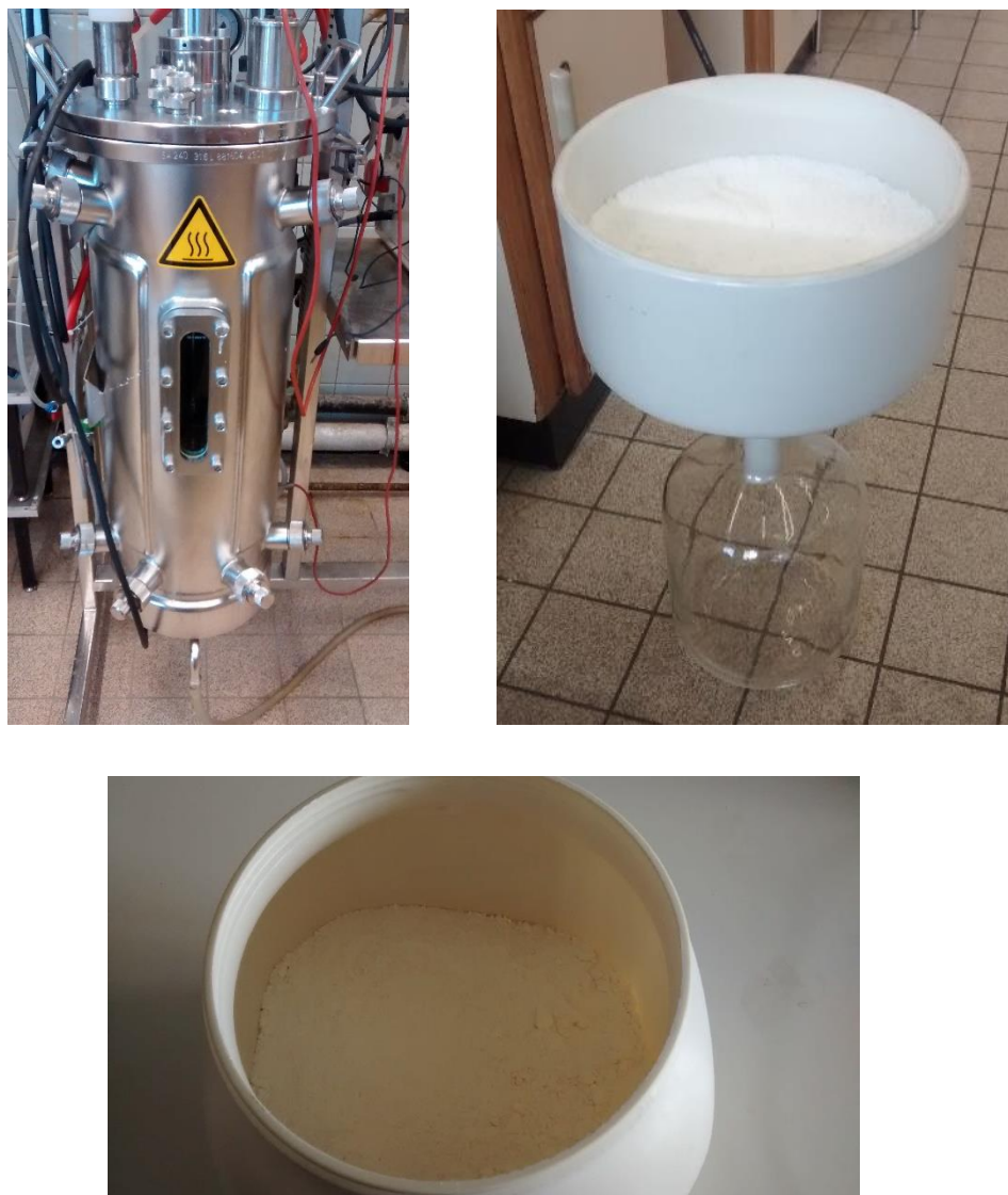
Figure IV.20: Reactor, purification and main result of the production at 10 L scale: 3 kg kojibiose with a purity higher than 99.8 %.
