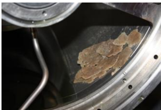
Figure 1: Precipitation in the Distillation Assembly Evaporator (Carter, 2010).
