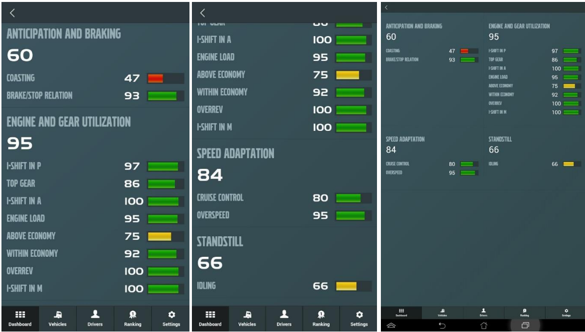
Figure 10: Parameters regarding fuel efficiency score of Dynafleet's mobile application on smartphone (left and center) and tablet (right)
