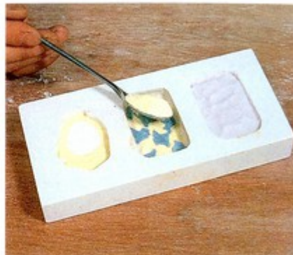
6. Charge the mold with colored glass, place it in the kiln, and fire.
