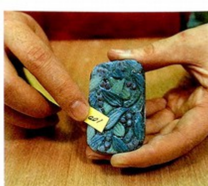
9. Grind with a diamond-grit (or wet/dry) sandpaper, and finish.
