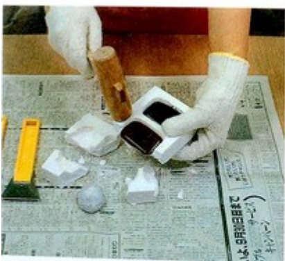
7. Release the mold after firing. Be careful not to tap on the glass.
