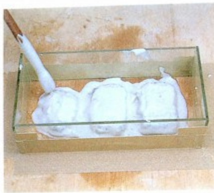
2. Construct a frame around the models and coat them with heat-resistant plaster mix.
