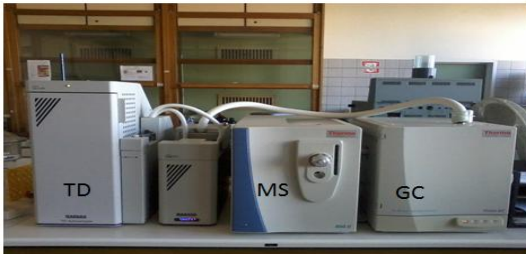
Figure 3.16: Thermal Desorption (TD)-Gas Chromatography (GC)-Mass Spectrometer (MS)
