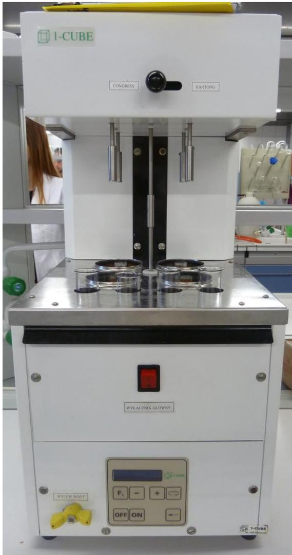
**Figure 4: Mashing machine: Mash Bath R-4, CUBE-1, Czech Republic**
