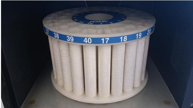
Figure 13: Rack for tubes of Mars Microwave
