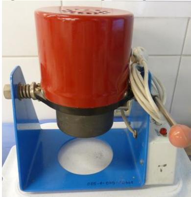
Figure 3: Electrical mixer, ZBPP type WZ-1
