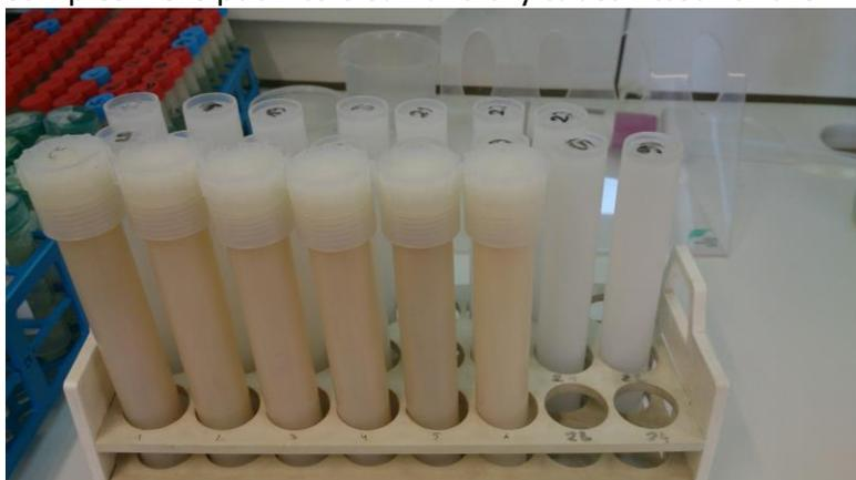
Figure 11: Tubes for digestion of organic compound with Mars Microwave
