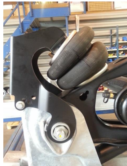
Figuur 6: Systeem om as volledig te liften
