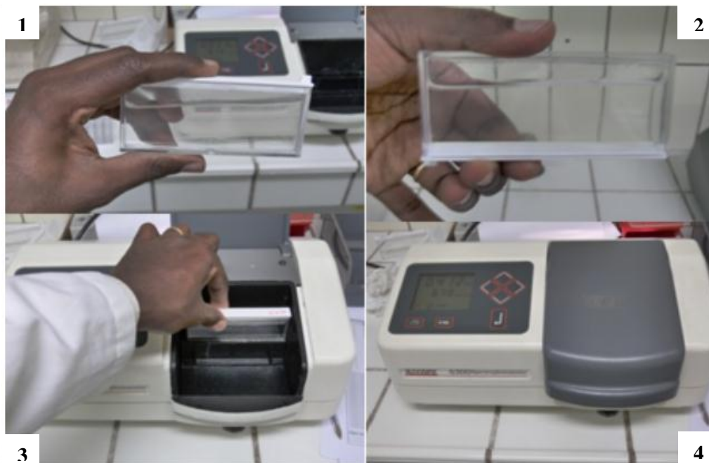
Fig. 11. Algal absorbance measurement. Gentle shaking of the algal culture by turning the test vial upside down to distribute the algae evenly (1&2) and measurement of light absorbance at 670 nm wavelength (3&4).
