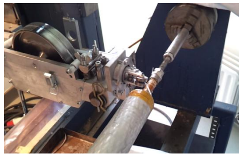
FIG.2: Filament winding with glass-fiber
