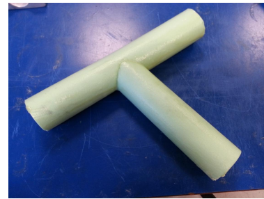
FIG.6: Polyurethane lug with latex
