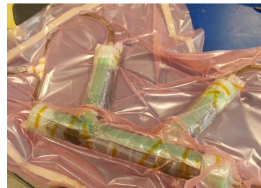
FIG.7: Draped lug in vacuum bag
