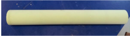
FIG.3: Mold out of polyurethane
