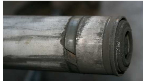
Figure 4: Adhesive wear of the rubber-aluminium contact due to lubrication problems
