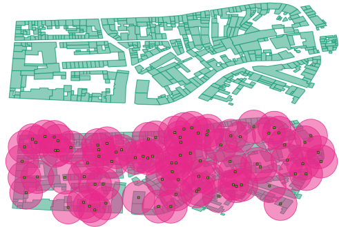
Fig. 2. Deployment of Mobile WiMAX femtocells in a given area. A bitrate of 5.7 Mbps and a bandwidth of 5 MHz is used.
