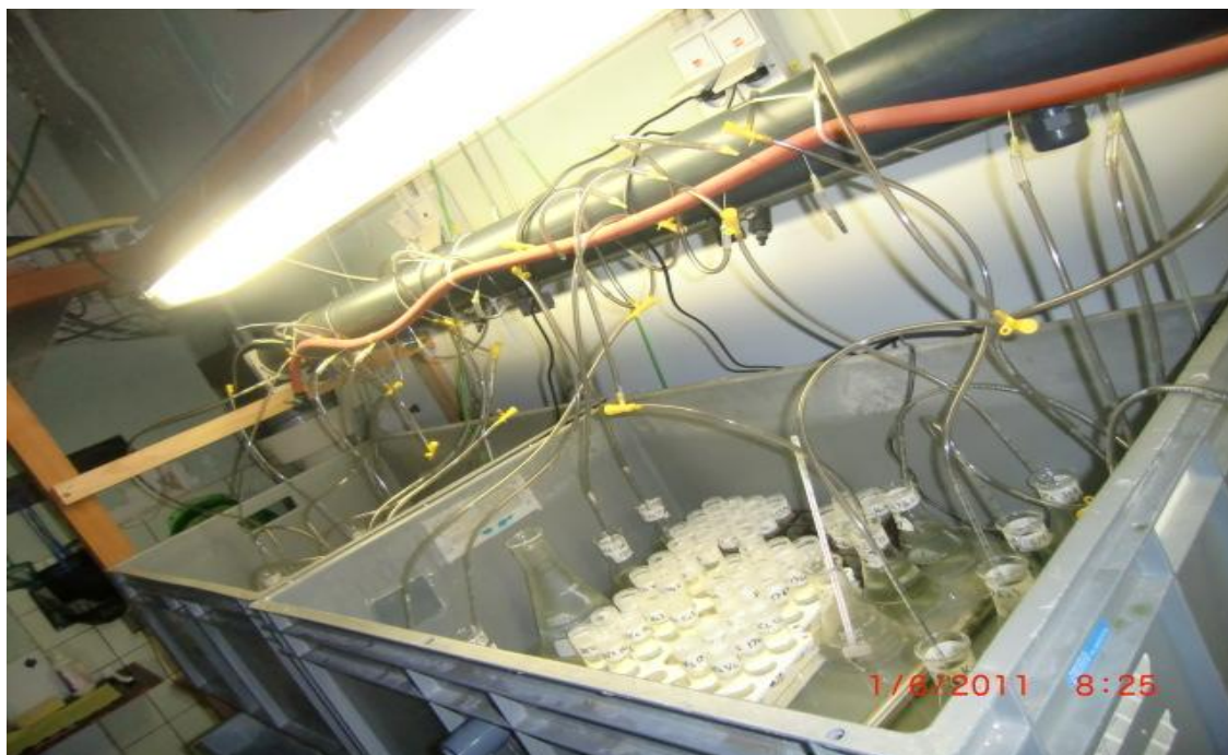
Figure 3. 7 Experimental set up showing falcon tubes and erlenmeyers immersed in a water bath, aerators and light tubes installed
