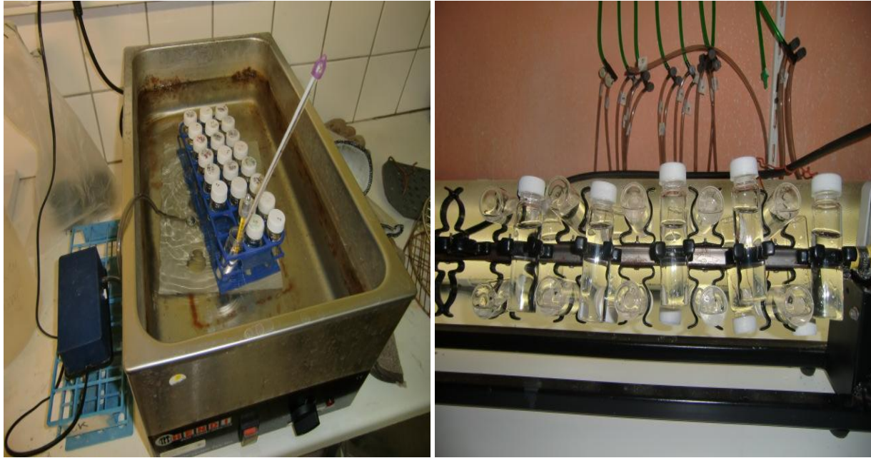
Figure 3. 8 Artemia heat shock experimental set-up. Left: heat shocking of Artemia in a water basin; right: glass tubes on rotator
