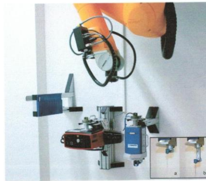
Figure 2. Tool stand with Virtobot in parking position. Left to right: needle holder, surface scanner and biopsy module. Bottom right: needle placement sequence with (a) needle retracted and (b) needle extended
