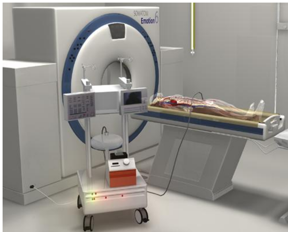
Virtobot setup (early and latest stage) in the Virtopsy examination room
