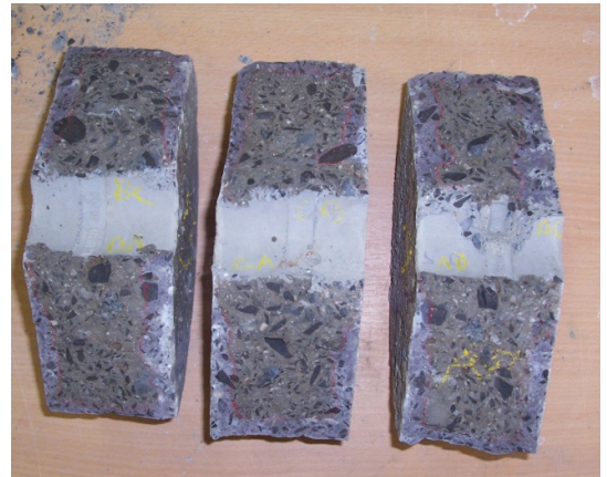
Figuur 3-12: Bepaling chloride-indringing
