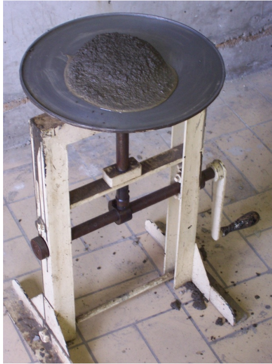
Figuur 3-24: Bepaling flow
