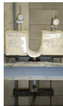
Figure 1: Construction sustained load
