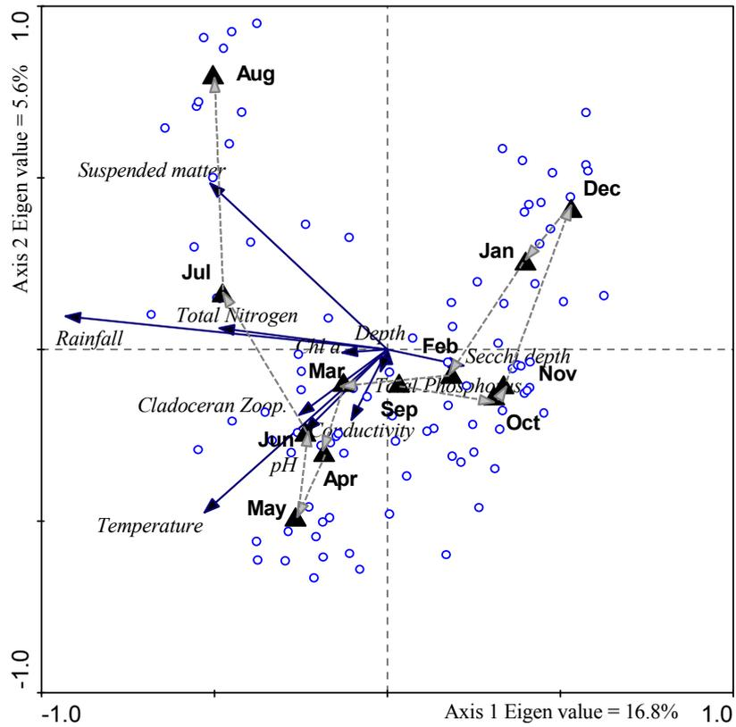
**Figure 3.2** First and second axis of a partial RDA on the response of environmental variables in function of month of the year, corrected for the influence of reservoir by including reservoirs as co-variables. Environmental variables are indicated by arrows, months by up-triangles, and samples by empty circles. Broken arrows indicate the sequence of sample collection. The first and second axes explain 16.8 and 5.6% of the total environmental variation, respectively.
