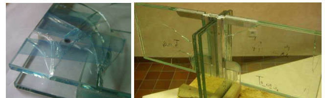
Fig. 7: cracks in the outer glass plate near the cut-away in the inner glass plate (left) and mounted prototypes of the clamp connection design from the second stage (right).
