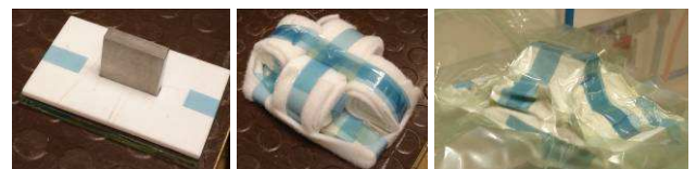
Fig. 3: Teflon mould (left), protected specimen (middle) and vacuum packed specimen (right).
