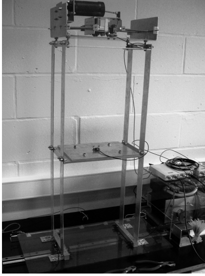
Fig. 2. Two-story frame with TMD on top
