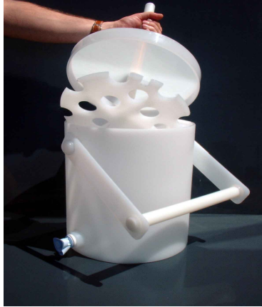
Figuur 3.9: Churn sample-splitter [16]
