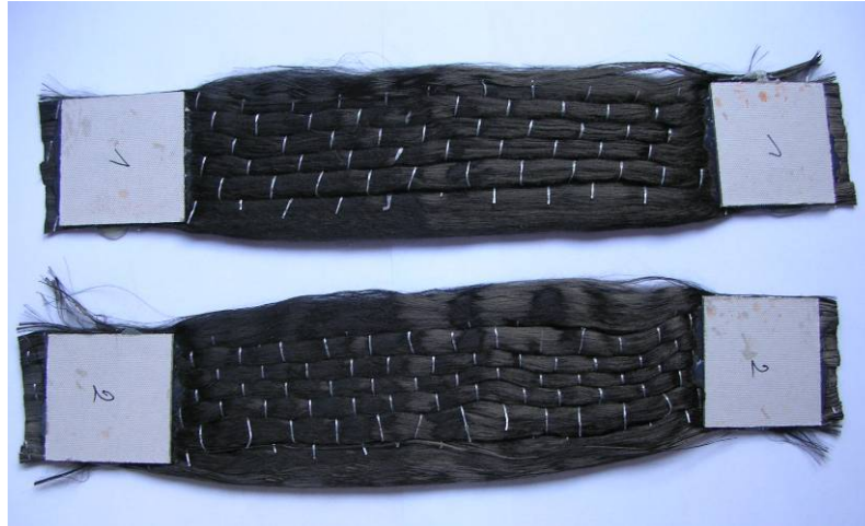
Figure 6.8: Embedded stripes of braid, after tensile test
