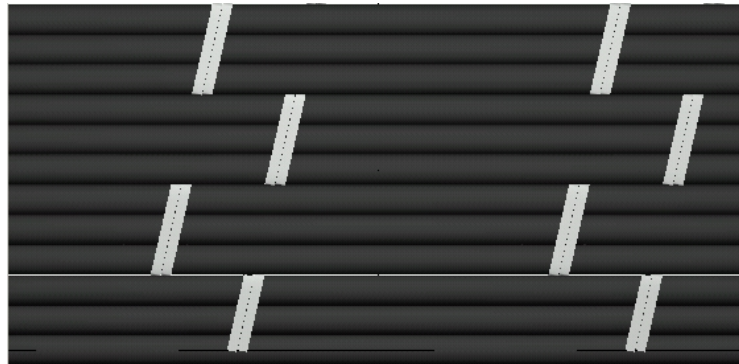
Figure 9.6: WiseTex model of compressed dry UD-braid
