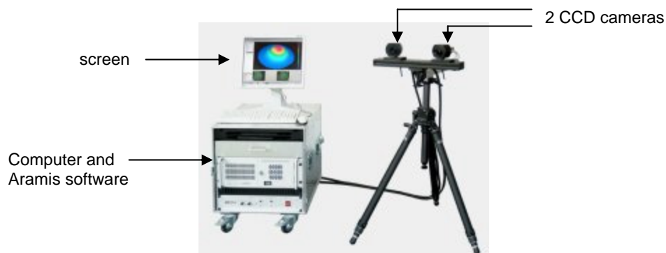
Figure 10.9: Aramis system, camera set-up [26]
