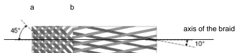
Figure 4.4: Braid with altering braiding angel (source: ITA)
