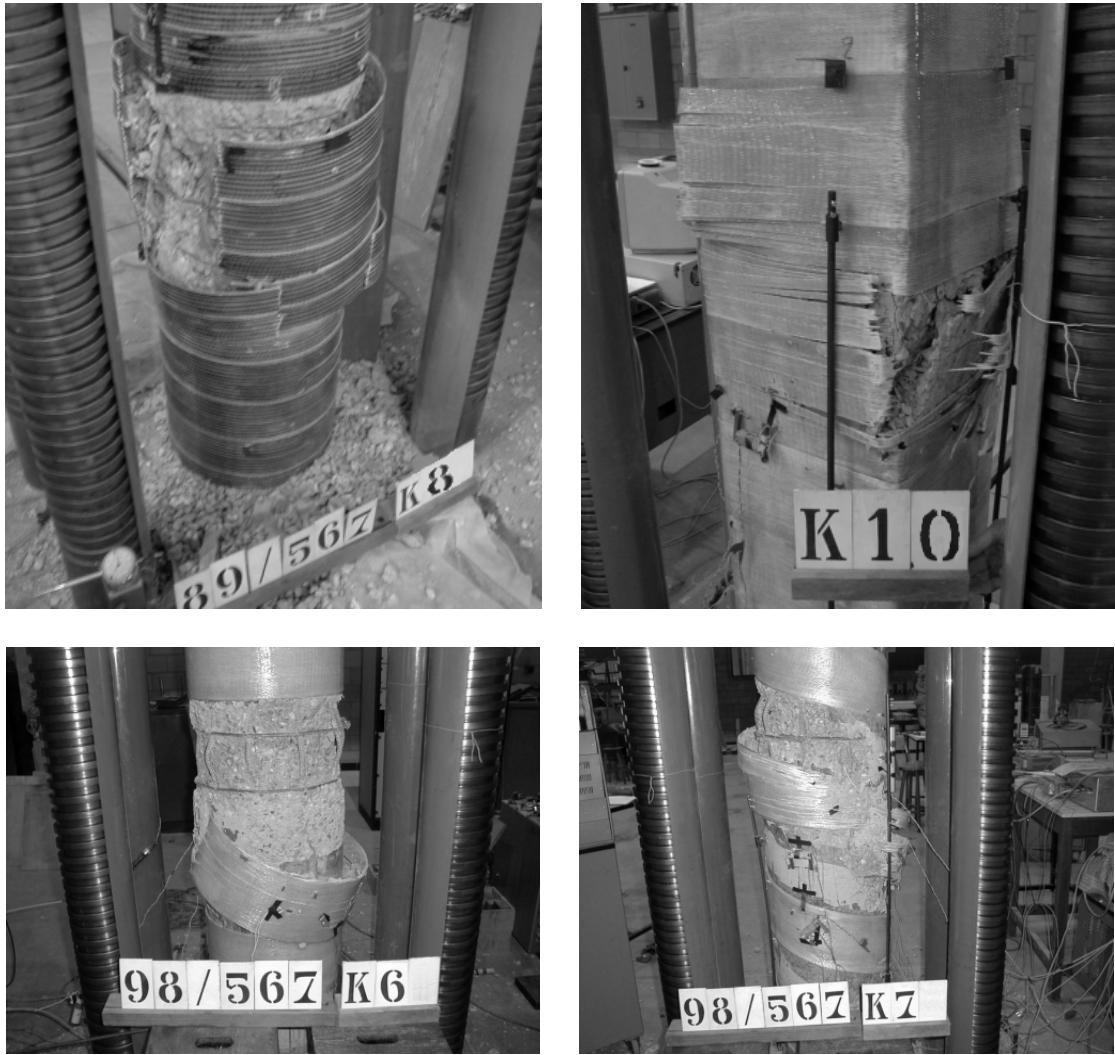
Fig. 6-7 Failure aspect of the confined columns
