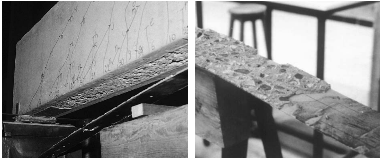
Fig. 3-3 Typical debonding failure mode of the strengthened beams
