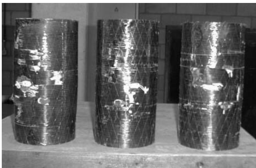
Fig. 6-3 Failure aspect of the wrapped cylinders C240nb
